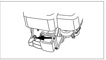
Figure 2. Typical Spark Plug Connection
